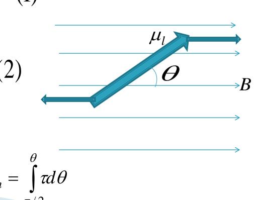
$$V_m = \int_{\pi/2}^{\theta} \pi d\theta = \mu_l B \int_{\pi/2}^{\theta} \sin \theta d\theta = -\mu_l B [\cos \theta]_{\pi/2}^{\theta} = -\mu_l B \cos \theta$$
